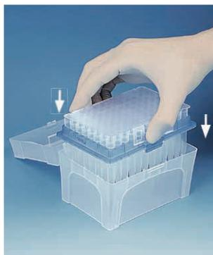
Insert the filled tip-tray perpendicularly from above into the previously sterilized TipBox until it locks into place.
