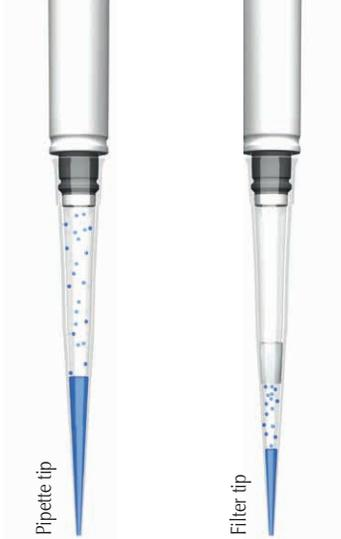
Non-self-sealing filter tips from BRAND have a PE filter that is free from chemical additives. Permeability is controlled by the combination of pore size and filter length, so that no aerosols can reach the pipette shaft. These filters function with consistent reliability. On the other hand, liquids can pass very slowly should they accidentally contact the filter. Since the filter does not
