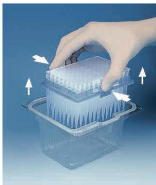
Press the long sides of the transfer aid together and continue pressing them together while withdrawing the tip-tray. Ensure that the holding straps for the transfer aid are correctly positioned.
