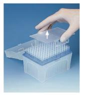
Remove the transfer aid from the mounting plate. Finished – all without tip contact!
