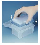
Insert the filled tip-tray perpendicularly from above into the previously sterilized TipBox until it locks into place.
