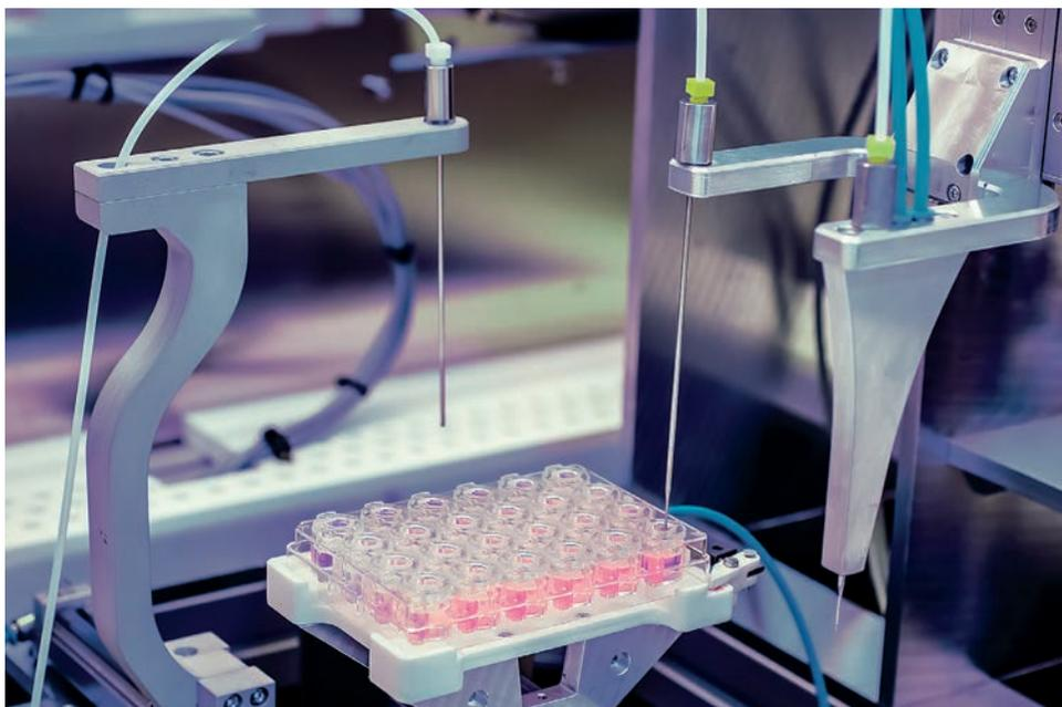
The described properties of the 6-well plate create even more benefit when combined with BRANDplates® Inserts with the Inlet Opening System (IOS) (patent pending). The medium in wells and inserts is interconnected by the IOS, so that it is possible to control medium level in both compartments simultaneously resulting in just 6 instead of 48 pipetting steps during medium exchange and when an air-liquid interface needs to be established.
